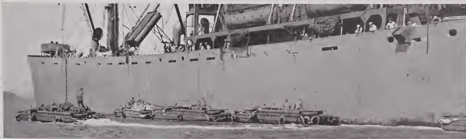
FIGURE 32. First operational use of DUKWs in discharging a Liberty ship, Noumea Harbor, New Caledonia, March 1943, 10 months after project was authorized by Director of OSRD.
